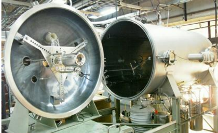
Figure 13. Vacuum test chamber for ion thrusters at LAP INPE, 1,5m of diameter and 3,0m of length
