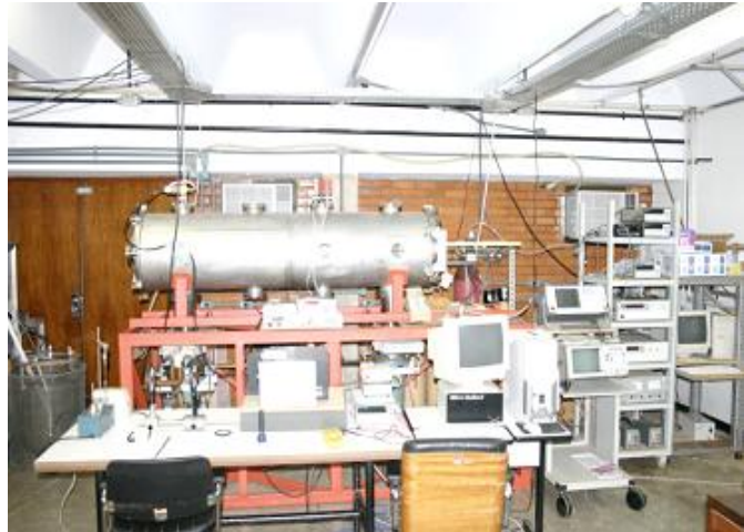
Figure 1. Plasma Physics Laboratory of UnB. View of Vacuum Chamber and Diagnostic Systems.
