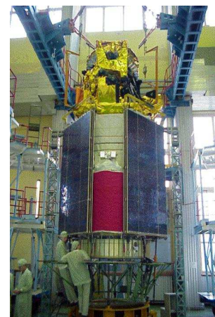
Figure 1. SESAT-1 satellite in the stowed configuration
