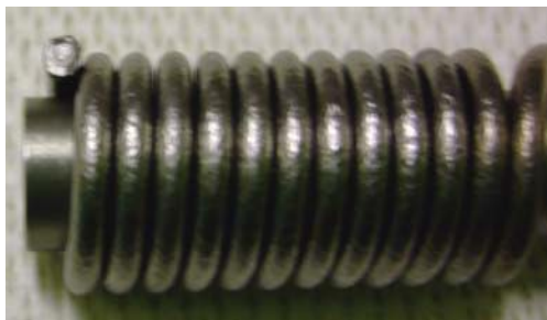
Fig. 1: Tantalum sheathed heater wire [3]
