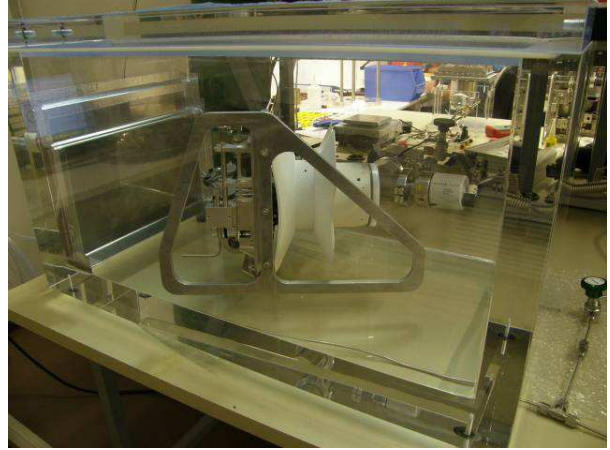
Figure 7. Photography of acrylic box for FCU integration welding process
