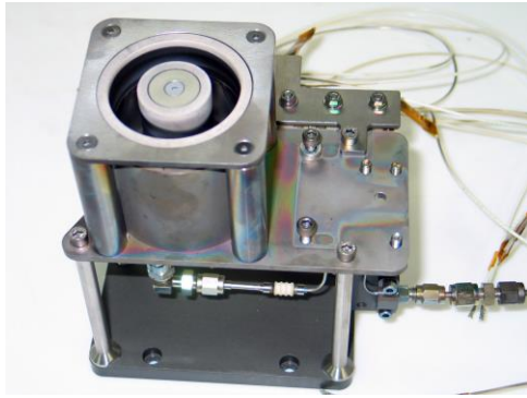
Figure 3. Experimental model of CAMILA Hall thruster (CAMILA-HT-55).
