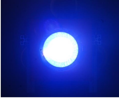
(a) Ar propellant at a mass flow rate 1.8 g/s and 3.75 kV charge voltage.
