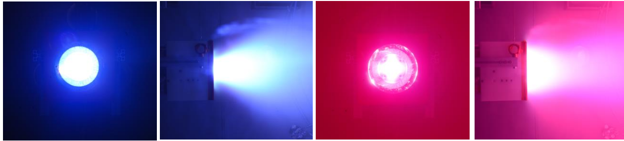
(a) Ar propellant at a mass flow rate 1.8 g/s and 3.75 kV charge voltage. (b) H 2 propellant at a mass flow rate 0.7 g/s and 2.25 kV charge voltage.
