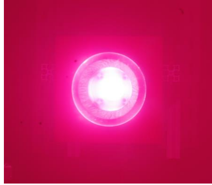
(b) H 2 propellant at a mass flow rate 0.4 g/s and 2.5 kV charge voltage.
