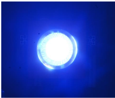
(c) Ar propellant at a mass flow rate 1.8 g/s and 4.00 kV charge voltage.
