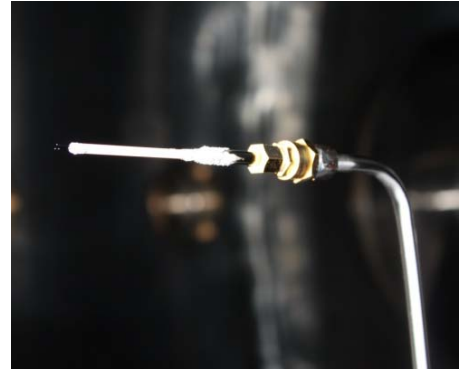
Figure 3. Langmuir probe design.
