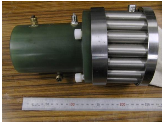
Figure 3. Photo of MPD thruster.
