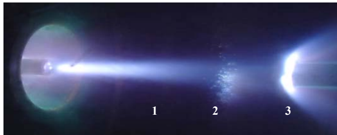
Figure 14. High power plasma flow interaction with micropowder and then with a sample. Pellets average dimension is 30 microns. Sample material is stainless steel. 1 – Initial plasma flow, 2 - pellets cloud, 3 – sample.
