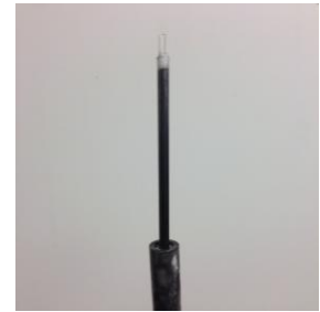
Figure 3. A translatable emissive probe. The alumina stem is coated to reduce secondary electron emission from the probe itself.
