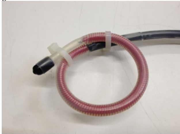
Figure 5. Photograph of a constructed Rogowski coil.
