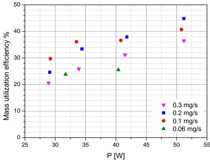
**Fig. 8 Mass utilization efficiency of ECR thruster vs MW power for different xenon mass flows.**
