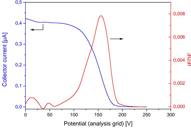
**Fig. 4 Typical ion current-voltage curve measured with the RPA (blue) in the thruster plume and corresponding IEDF (red).**
