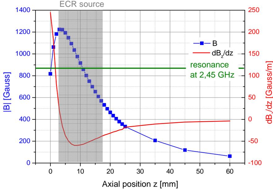
**Fig. 2 Axial magnetic field strength  $B_z$  and magnetic field gradient  $dB_z/dz$  in the electron cyclotron source and the magnetic nozzle.**
