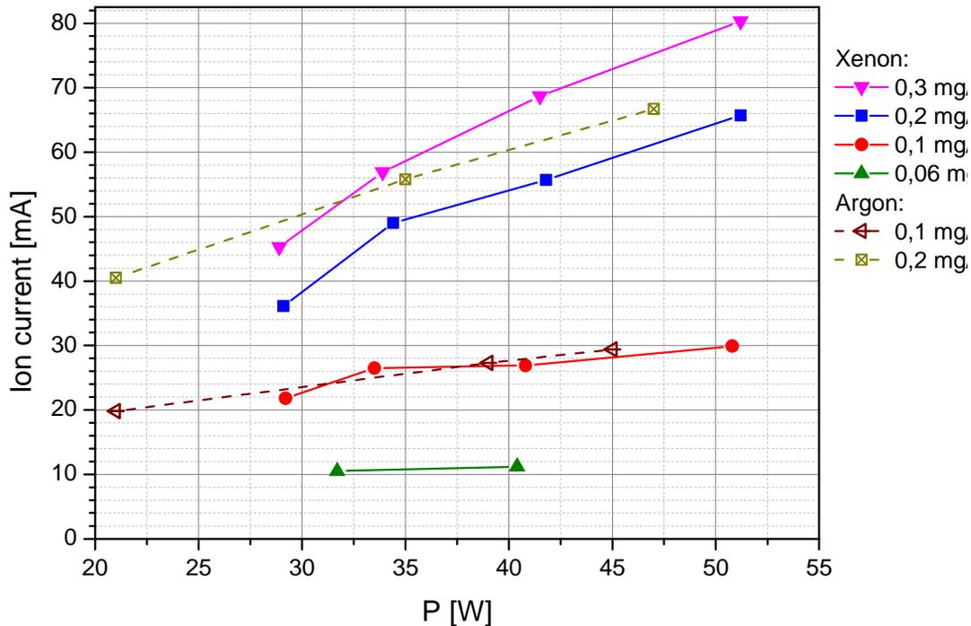
**Fig. 7 Total ion current vs MW power for xenon (left) and argon (right). Flow rates are in mg/s.**
