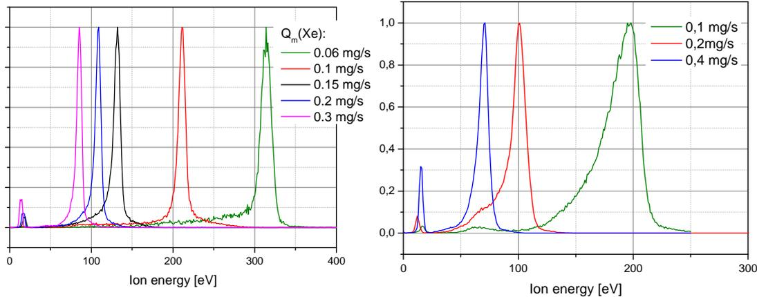
**Fig. 9 Dependence of IEDF (normalized) on the xenon mass flow (left) and on the argon mass flow (right).**
