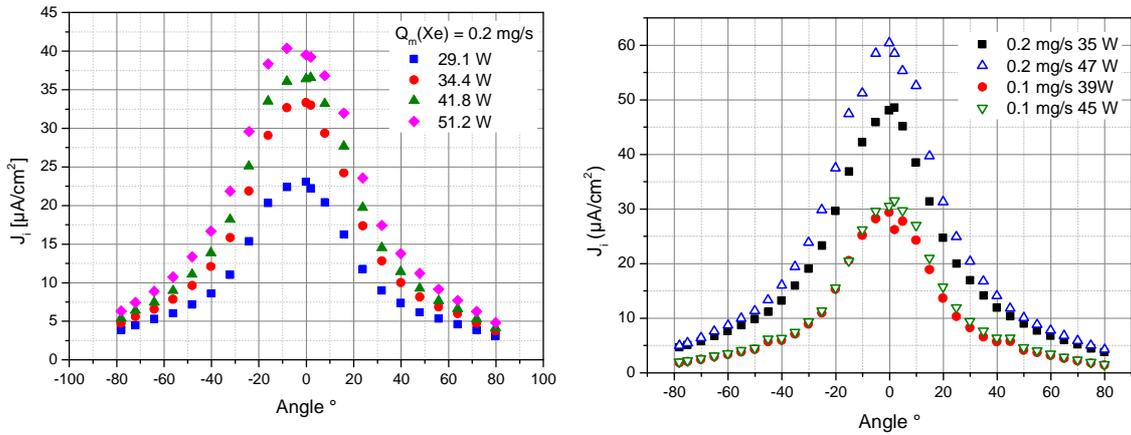
**Fig. 6 Angular profile of the ion current density for a xenon (left) and argon (right).**
