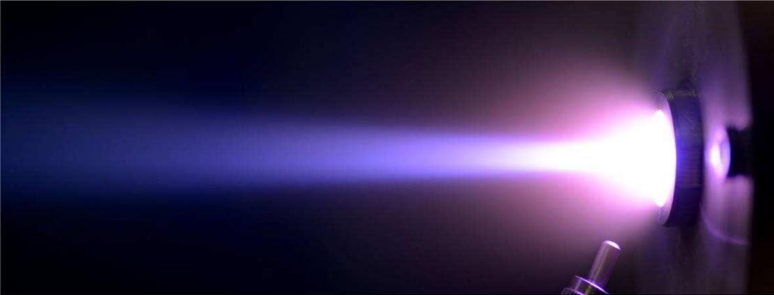
**Fig. 5 View of ECR thruster plume in argon.**
