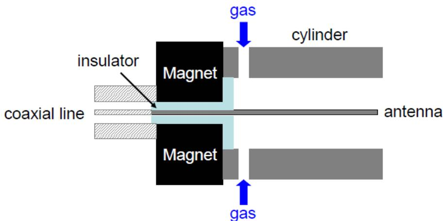
**Fig. 1 Schematic diagram of the ECR source.**
