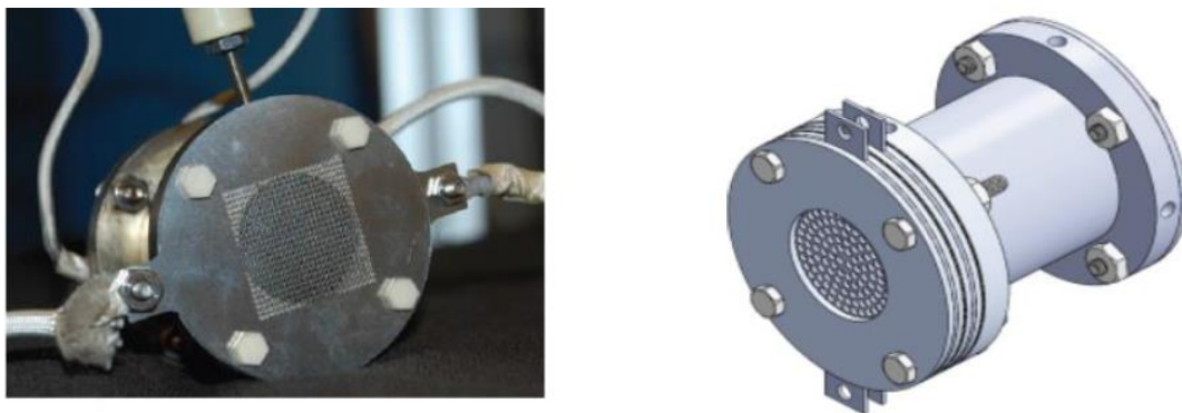
Figure 4. Electron Gun. Figure shows an electron gun with high transparency grid used for SEE tests along with a 3D model
