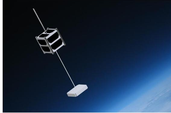
**Figure 11. MiTEE mission spacecraft concept showing the CubeSat deploying the endmass.** Here, the tether is only deployed a short distance.
