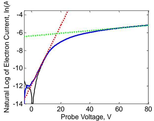
**Figure 8. The  $\ln(I_e)$ –V characteristic for the 0.5-cm spherical probe.** The natural log of the probe current is shown in black. The electron current (ions subtracted) is shown in blue. The red line is the best fit line for the electron retardation region and the green line is the best fit line for the electron saturation region.
