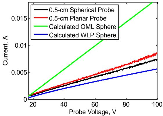
**Figure 9. The I–V characteristic for the 0.5-cm spherical probe and the 0.5-cm planar probe compared to current calculated by the OML and WLP models.**
