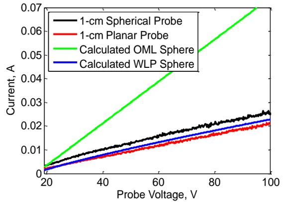
**Figure 10. The I–V characteristic for the 1-cm spherical probe and the 1-cm planar probe compared to current calculated by the OML and WLP models.**
