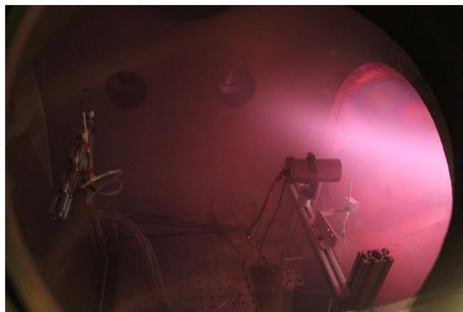
**Figure 6. The probes in the high speed plasma plume.**
