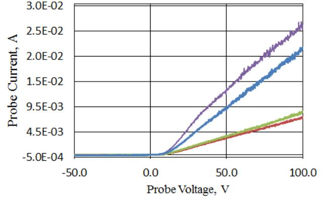
**Figure 7. The current-voltage characteristic for each type of probe.** The characteristics for the 1-cm spherical probe (purple), the 1-cm planar probe (blue), the 0.5-cm spherical probe (red), the 0.5-cm planar probe (green).
