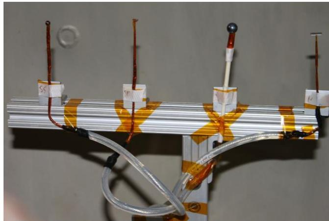
**Figure 5. Probes mounted in the vacuum chamber.** From left to right, there is the 0.5-cm spherical probe, the 0.5-cm planar probe, the 1-cm spherical probe, and the 0.5-cm planar probe.
