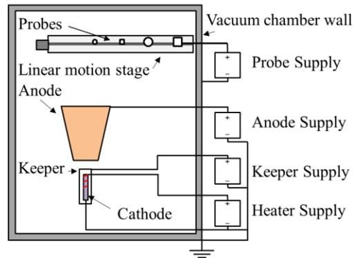
**Figure 3. Setup of the vacuum chamber showing the hollow cathode plasma source and the probes.**
