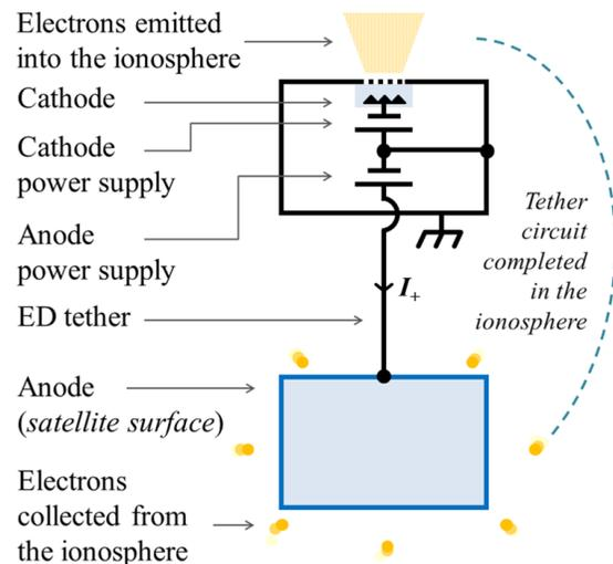
Figure 2. A diagram of the system concept. The core components of the tether propulsion system are shown. In a possible alternative configuration, the anode and cathode power supplies would be located on separate satellites, though similarly connected.
