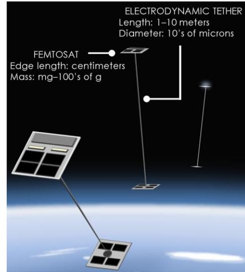
Figure 1. An illustration showing the concept of ED tethers connecting pairs of femtosatellites in a maneuverable, coordinated fleet.<sup>7</sup>
