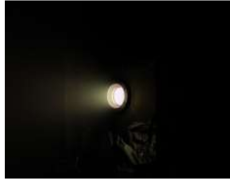
Figure 1. RIT10-EBB thruster running with N 2 +O 2 .
