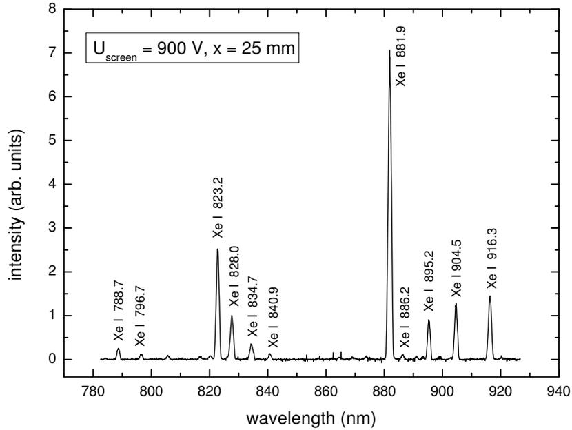
Figure 2. NIR spectrum in the plume of the ISQ40RF ion source at an axial distance 25 mm downstream the exit plane, with  $U_{screen}=900$  V,  $P_{RF}=45$  W. All indicated emission lines are associated to neutral xenon.
