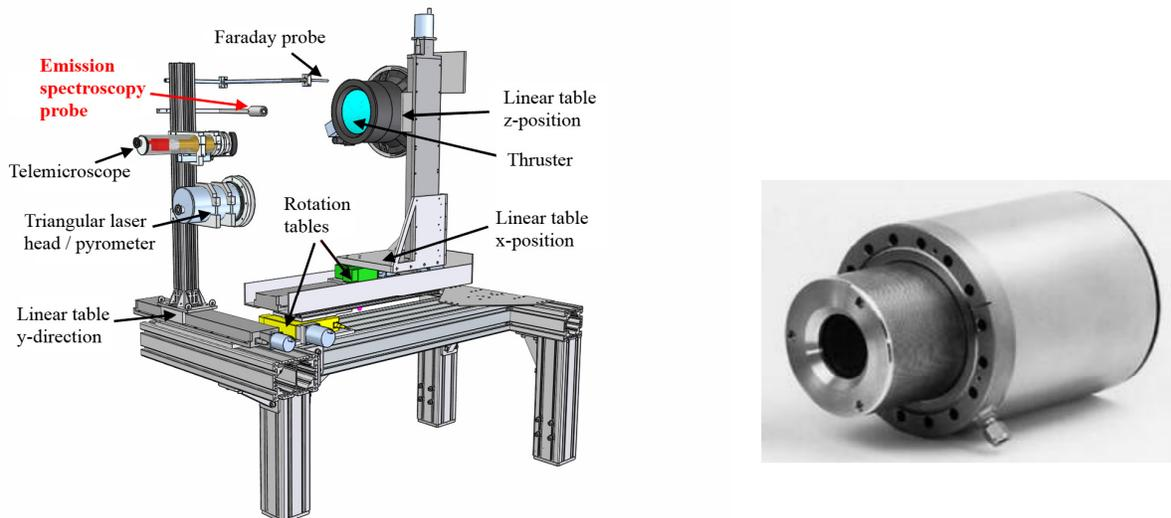
Figure 1. Left: Diagnostic instrumentation including the emission spectroscopy probe on the 5-axis positioning system of the AEPD complex.<sup>4</sup> Right: The ISQ40RF ion source.
