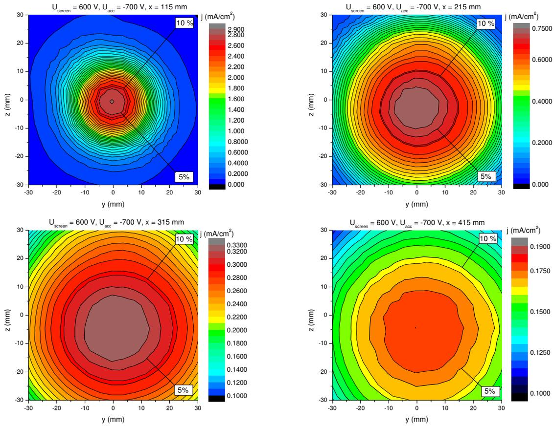
Figure 4. Exemplary Faraday mapping profiles in the plume of the ISQ40RF ion source, without beam neutralization,  $U_{screen}=600$  V,  $P_{RF}=40$  W. Within marked areas, the current density differs less than 5 or 10% with the central value, respectively.
