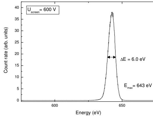
Figure 5. Ion energy distribution at 132 amu measured on the central thruster axis, same operation condition as in Figure 4.
