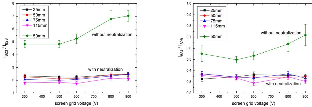
Figure 3. Emission line ratios measured at several axial distances, in dependence of the screen grid voltage. All measurements are integrated emissions over the line-of-sight. The measurements at axial distance of 50 mm are shown with and without beam neutralization.
