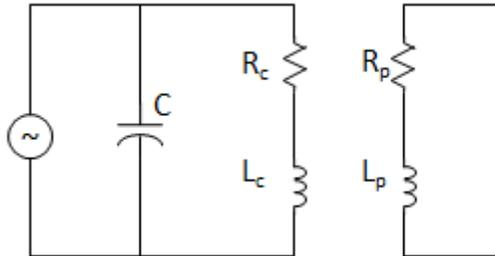
**Figure 2. Representation of the transformer model for the ICP.**
