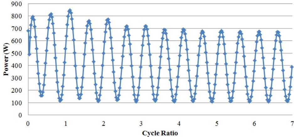
Figure 5. First 7 cycles of power deposition vs. cycle ratio.
