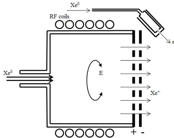
Figure 1. Schematic of an RF ion thruster
