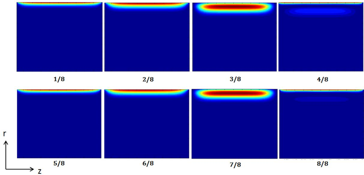
Figure 6. Cycle ratio and power deposition. The fractions denote the cycle ratio within one full RF cycle.
