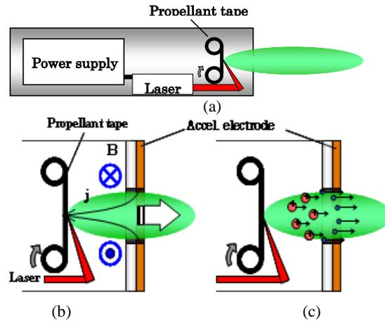
**Figure 1. Schematics of laser ablation thrusters**
