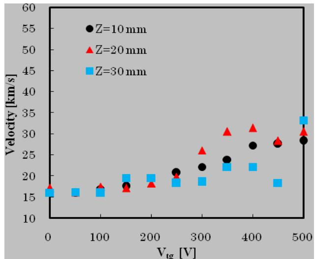
**Figure 6.** Variations of ion velocity of thruster A with acceleration voltages measured with Faraday cup placed at 80 mm away from the target.
