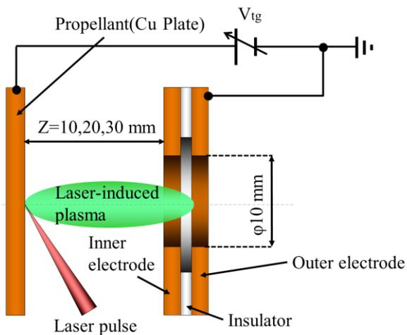
Figure 3. Laser-electrostatic hybrid thruster A
