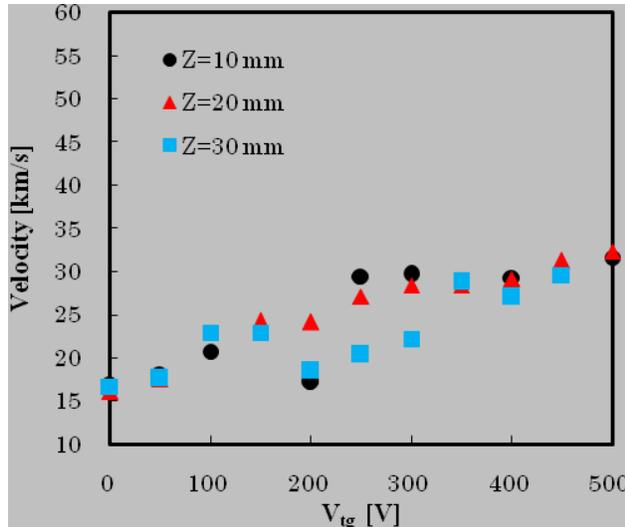
**Figure 5.** Variations of ion velocity of thruster A with acceleration voltages measured with Faraday cup placed at 50 mm away from the target.
