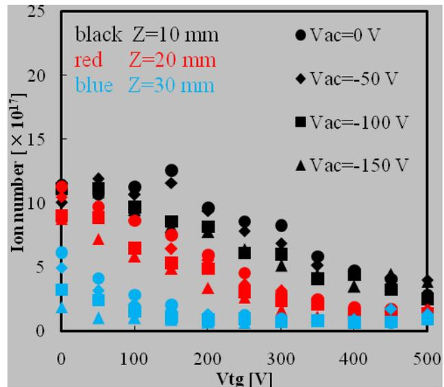
**Figure 10.** Variations of ion number of thruster B with acceleration voltages measured with Faraday cup placed at 50 mm away from the target.
