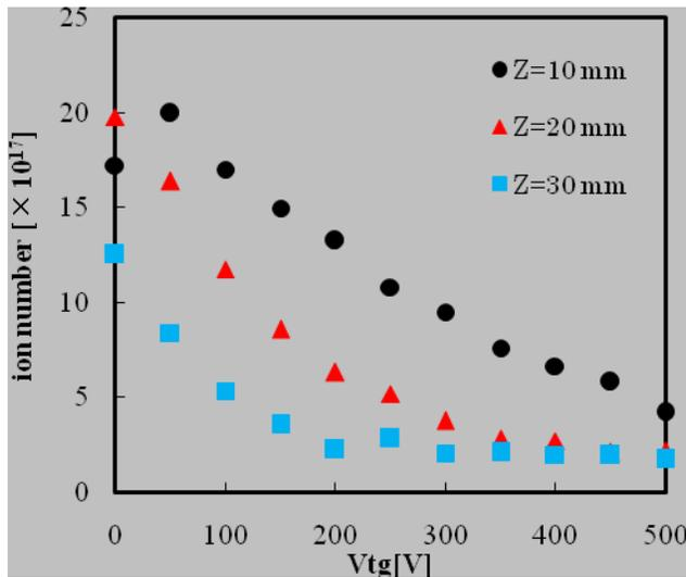
**Figure 7.** Variations of ion number of thruster A with acceleration voltages measured with Faraday cup placed at 50 mm away from the target.
