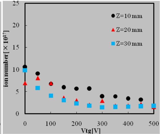
**Figure 8.** Variations of ion number of thruster A with acceleration voltages measured with Faraday cup placed at 80 mm away from the target.
