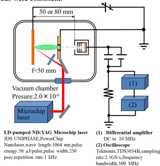
Figure 2. Experimental setup
