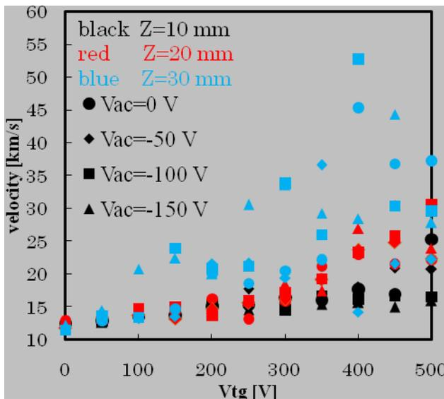
**Figure 9.** Variations of ion velocity of thruster B with acceleration voltages measured with Faraday cup placed at 50 mm away from the target.
