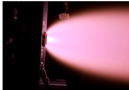
Figure 11. Picture of hollow cathode operation with outer injection.
