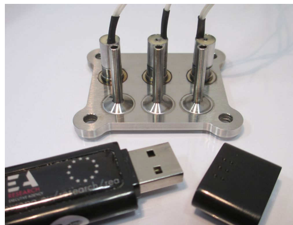
Figure 2. \mu FCU EQM 02 in comparison to the size of an USB stick
