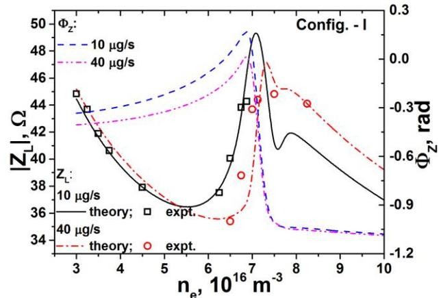
Figure 10. Variation of calculated  $|Z_L|$  and  $\Phi_Z$ , and experimental  $|Z_L|$  with  $n_e$  in Config. – I.
