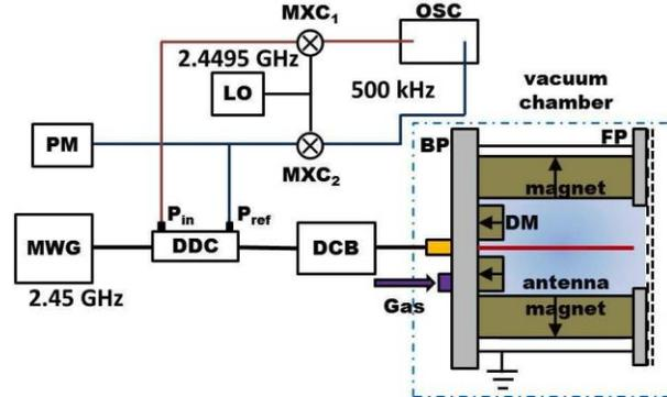
Figure 5. Reflection coefficient measurement setup.
