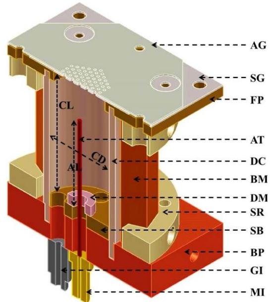
Figure 1. Design schematic of the ion thruster.
