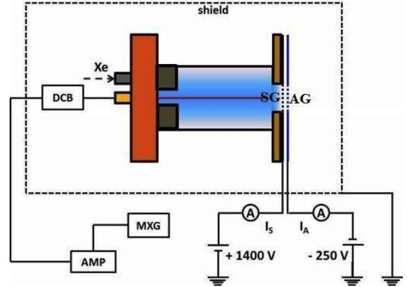
Figure 3. Setup for ion beam extraction.
