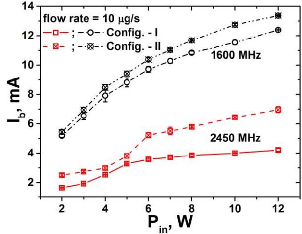
Figure 4. Variation of extracted ion beam current with input power.
