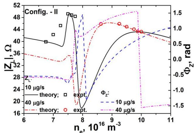
Figure 11. Variation of calculated  $|Z_L|$  and  $\Phi_Z$ , and experimental  $|Z_L|$  with  $n_e$  in Config. – II
