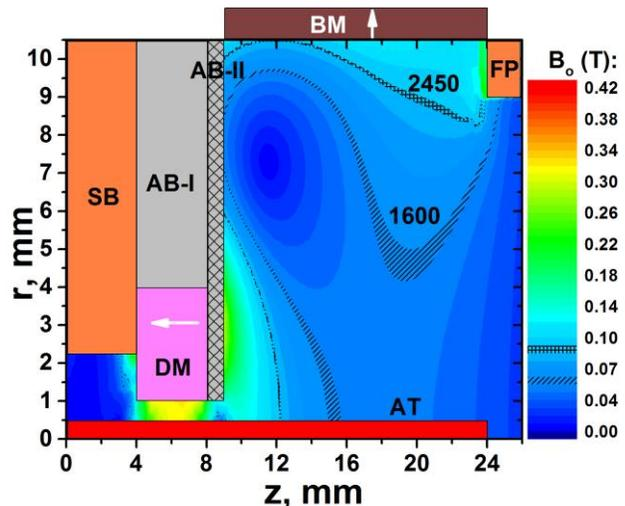
Figure 2. Contour plot of the magnitude of magnetic field in the axial plane.
