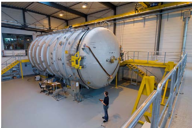
Figure 1. Vacuum chamber of the electric propulsion test facility at DLR Goettingen.
