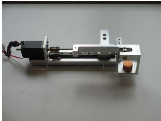
Figure 9. Gravimetric calibration mechanism with three stacked copper weights (cylindrical copper-colored pieces on the right).
