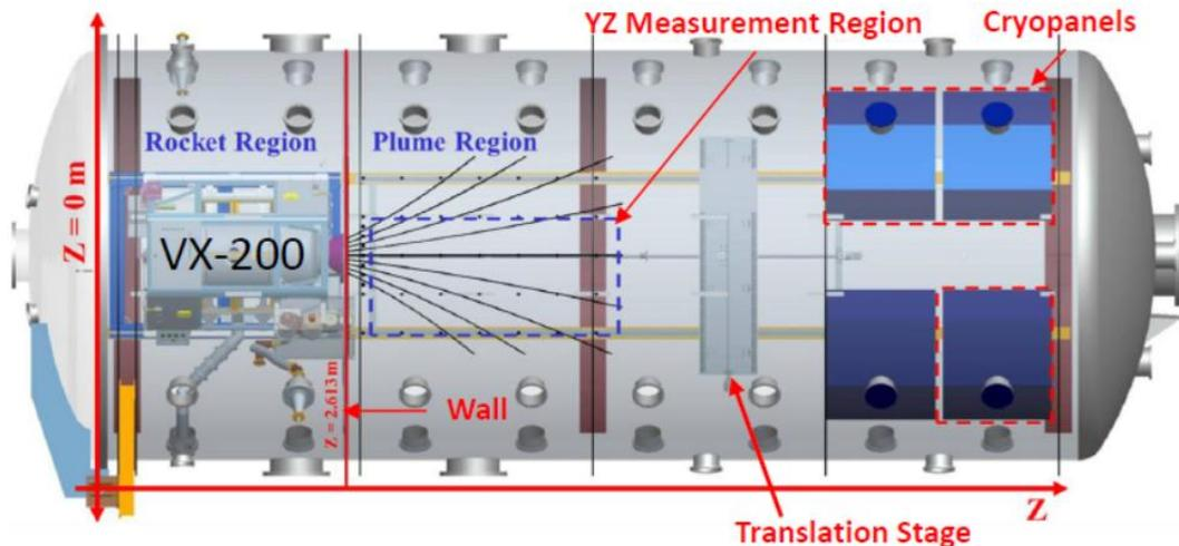
Figure 2. Schematic of the 10 m long x 4.3 m diameter vacuum chamber and the VX-200<sup>™</sup> engine
