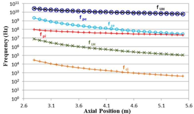
**Figure 5. Natural frequencies along the plume axis in the probe measurement region:  $f_{ci}$  (ion cyclotron),  $f_{LH}$  (lower hybrid),  $f_{pi}$  (ion plasma),  $f_{ce}$  (electron cyclotron),  $f_{pe}$  (electron plasma),  $f_{UH}$  (upper hybrid)**
