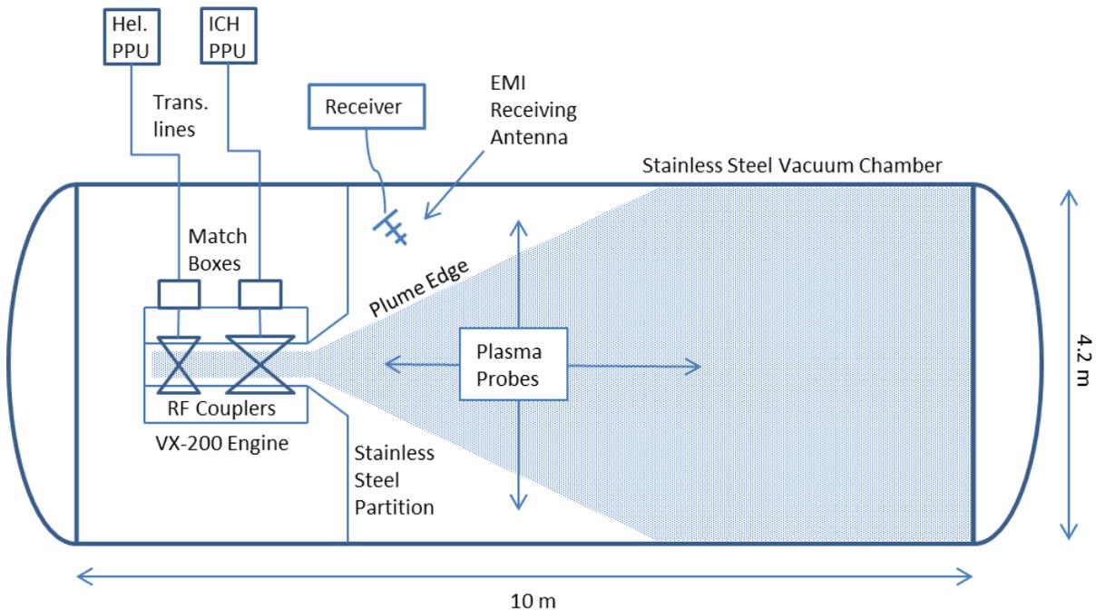
**Figure 3. Conceptual Schematic of Receiving Antenna Placement for Plume EMI Study. Possible sources of EMI include: RF PPUs, matching networks, transmission lines, rocket core, and the plasma plume. This paper focuses on measuring and modeling EMI from the plume.**
