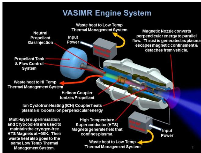
Figure 1. Schematic diagram of a VASIMR<sup>®</sup> System
