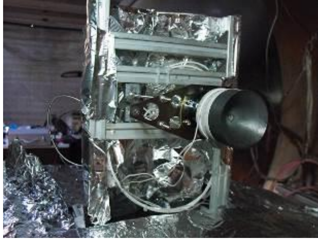
Figure 7. T6 HCTs mounted on the thrust balance at AER
