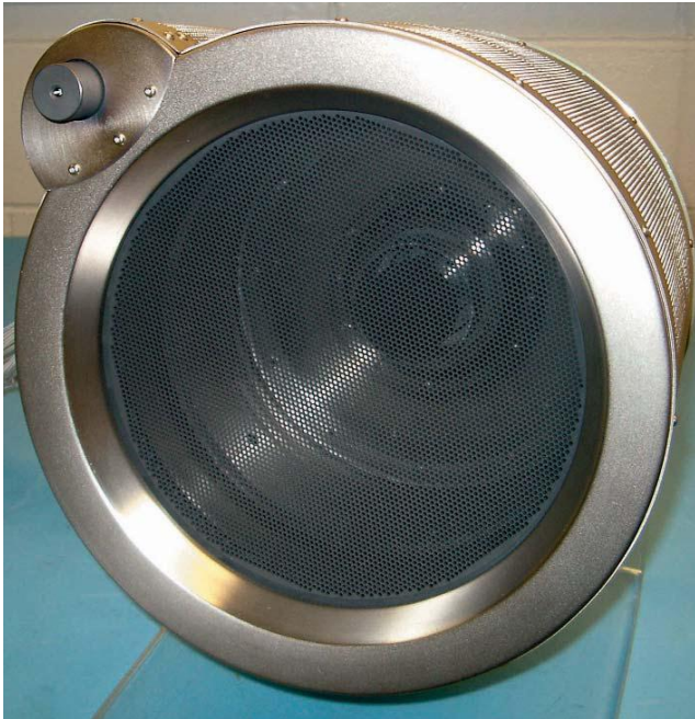
Figure 4. T6 Electron-Bombardment Ion Thruster (reproduced by permission of QinetiQ)
