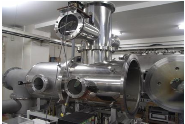
Fig. 6. PPT experimental system installed in vacuum chamber
