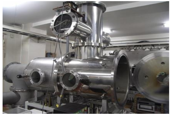
Fig. 6. PPT experimental system installed in vacuum chamber
