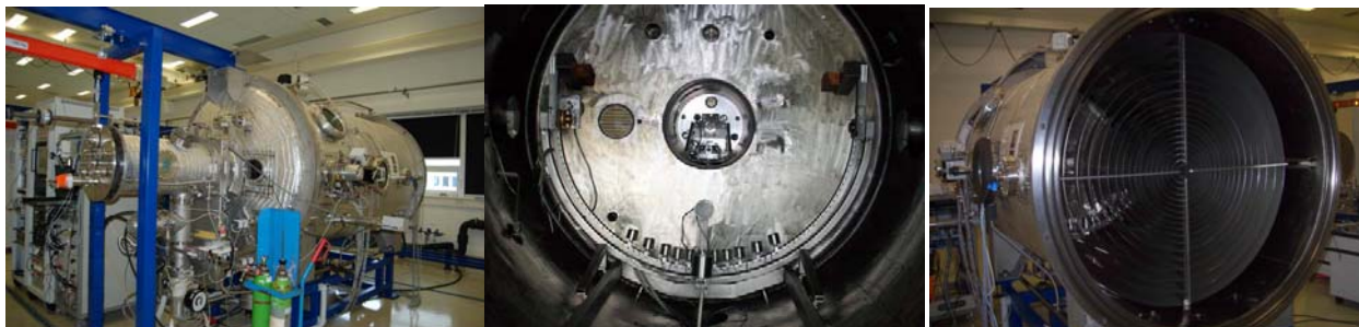
Figure 9: EPL GIGANT facility with its diagnostic system of 11 Faraday Cups and the target
