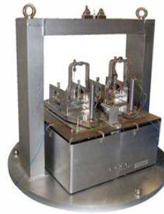
Figure 4. EPL MicroNewton Thrust balance developed in collaboration with the National Physics Laboratory (UK) and its achieved performance.
