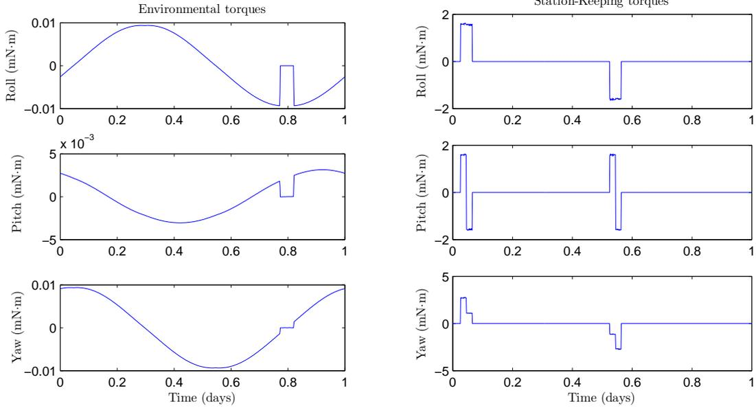
Figure 3. Disturbance torques:  $\tau_e$ (left),  $\tau_{sk}$ (right)
