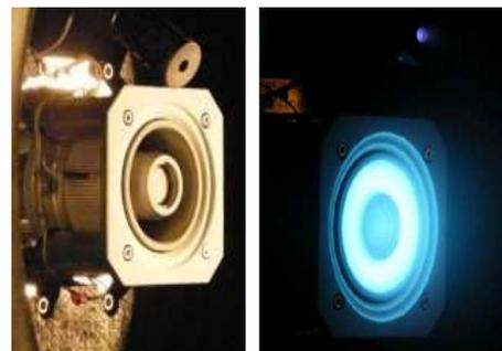
**Figure 2. Thruster PPS®X00 prototype n°1.** Thruster firing during initial validation test Designed for 300W, it shows anode efficiencies up to 40%<sup>5</sup>
