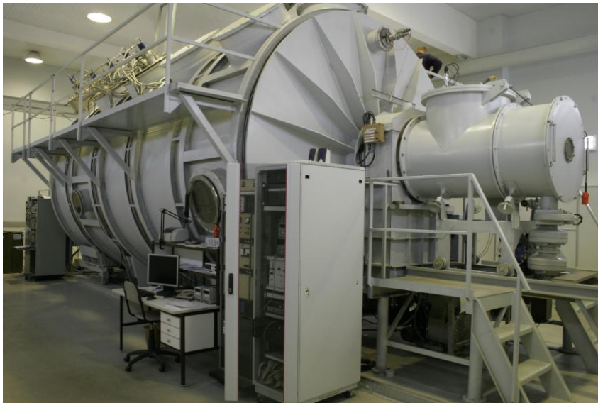
Figure 3. Appearance of KVVU-90 vacuum chamber.
