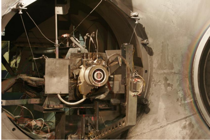
Figure 2. Thruster KM-60 in the KVVU-35 facility while setting diagnostic systems.
