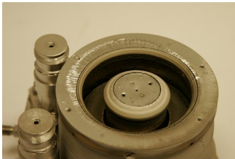
Figure 15. Appearance of KM-60 thruster after lifetime test.
