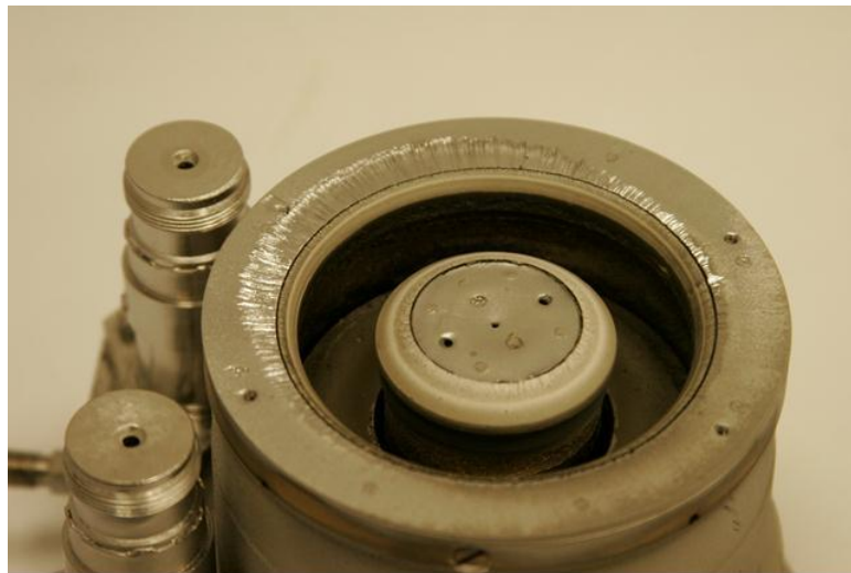
Figure 15. Appearance of KM-60 thruster after lifetime test.
