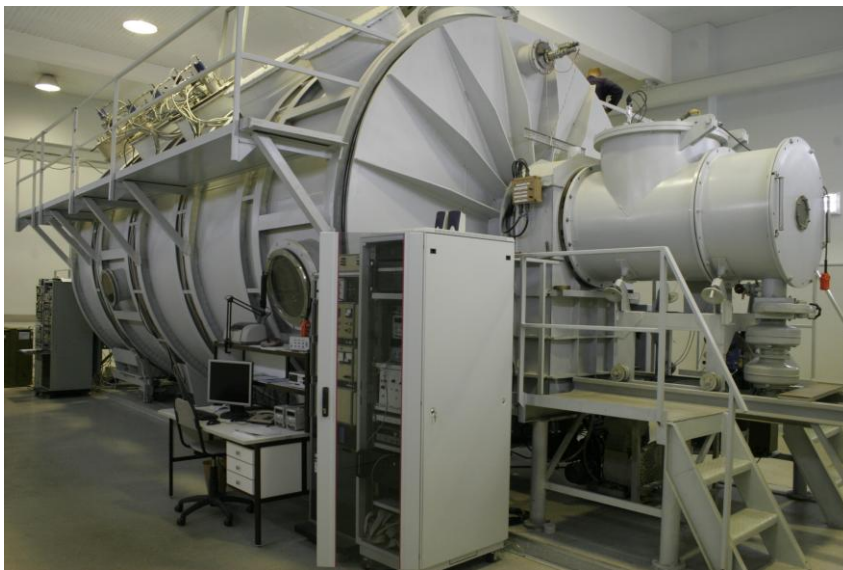
Figure 3. Appearance of KVVU-90 vacuum chamber.
