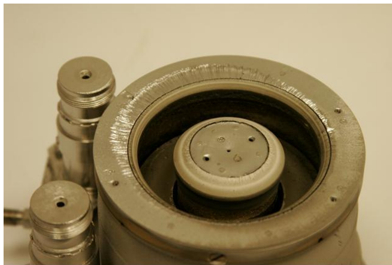
Figure 15. Appearance of KM-60 thruster after lifetime test.
